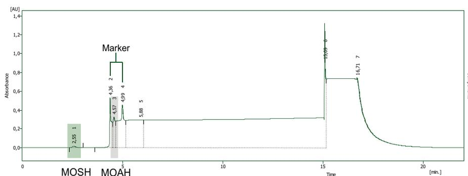
Figure 2: LC chromatogram of a contaminated rice sample: Peak 1 (2.55 min, MOSH), peak 3 (4.57 min, MOAH), peaks 2,4 are marker compounds
