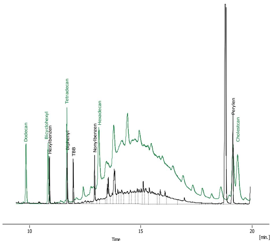
Figure 3: Parallel injections of the LC-MOSH fraction (green) and LC-MOAH (black) fraction (as highlighted in Fig. 2) into the GC
