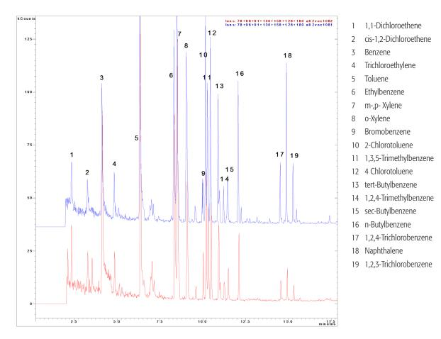
Figure 6: Chromatographic Comparison of PAL 95 µm Carbon WR Fiber (blue) and Brand X Carboxen® fiber (red).
