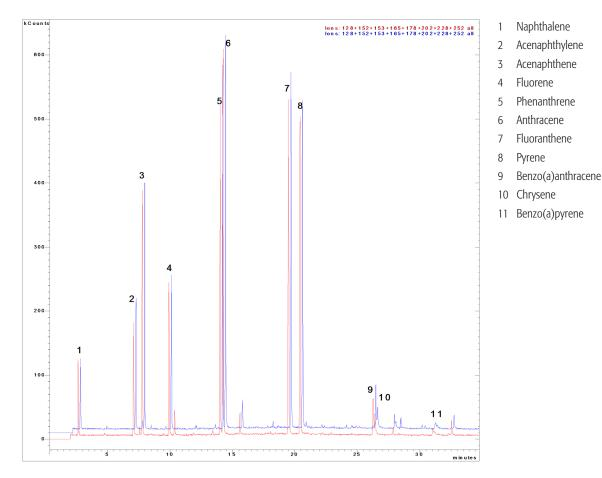
Figure 1: Chromatographic Comparison of PAL Fiber PDMS 7 µm (blue) and Brand X Fiber (red).
