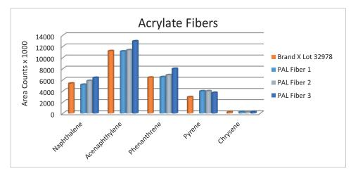
Figure 4: Quantitative Comparison of PAL 85 µm Acrylate Fiber and Brand X Fiber for Five selected Target Molecules.
