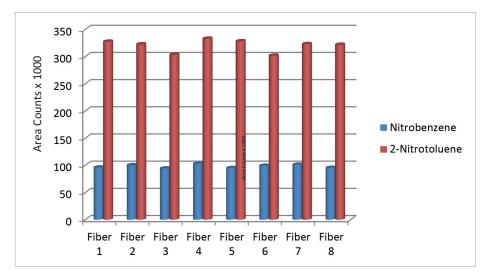
Figure 8: Fiber to Fiber Reproducibility Test.
