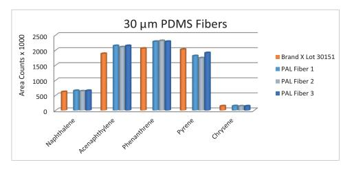
Figure 3: Quantitative Comparison of PAL 30 µm PDMS Fiber and Brand X Fiber for Five selected Target Molecules.
