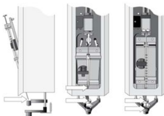
Figure 38. Installing and Removing a Syringe for Liquid Injections
