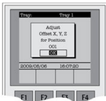
Figure 29. Adjusting “Offset X,Y,Z” for Tray Position 001
