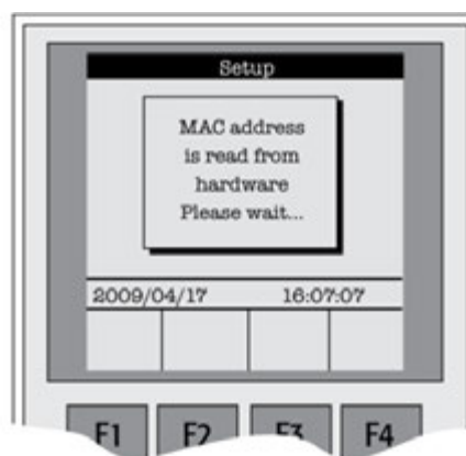
Figure 43. Reading the MAC Address from the Ethernet Communication Port
