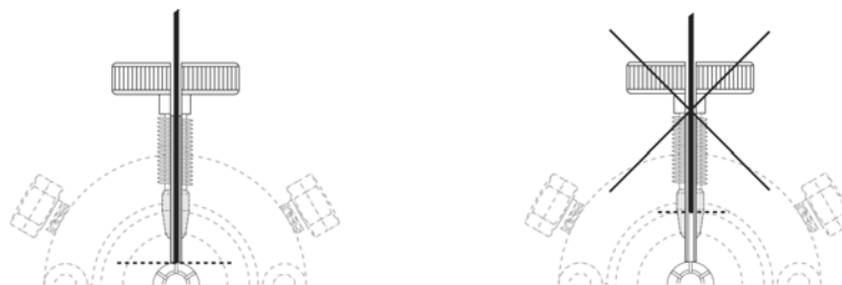
Figure 42. Correct and incorrect Valve Needle Penetration Depth.
