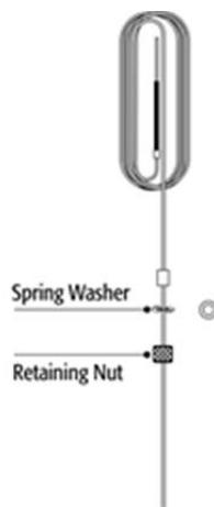
Figure 16A. Using Spring Washer to hold Retaining Nut in Position.
