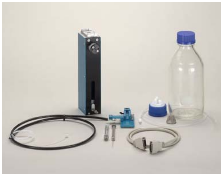
Figure 1. PAL Dilutor General System Overview
