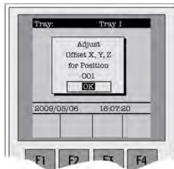
Figure 27. Adjusting “Offset X,Y,Z” for Tray Position 001
