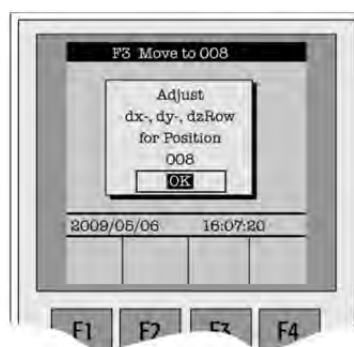
Figure 28. Adjusting Row Inclination at Second Tray Corner Position
