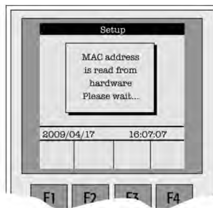
Figure 48. Reading the MAC Address from the Ethernet Communication Port
