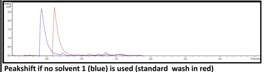
Solvent 1 equals eluent A to avoid any effect on the retention (e.g. shorter retention-time).
