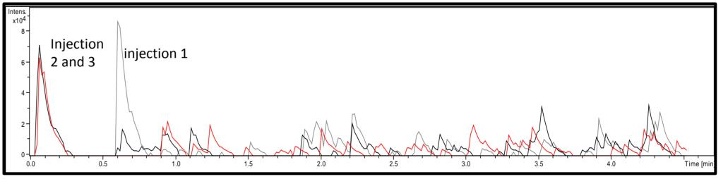
The regeneration time is evaluated by comparing 3 consecutive injections. The regeneration is too short as soon as the signals don't overlap. This is buffer, column and flow dependent.
