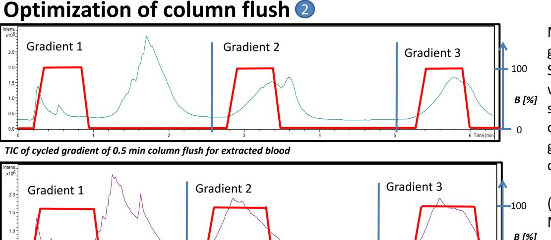
Matrix is injected and the gradient is run in cycles. Several runs are carried out with shorter flushing times. As soon as significant effects are observed in the 2<sup>nd</sup> and 3<sup>rd</sup> gradient, the method is considered as too short.
