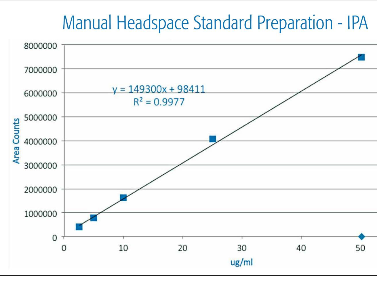
Figure 3: The standard curve for IPA headspace standards prepared manually.
