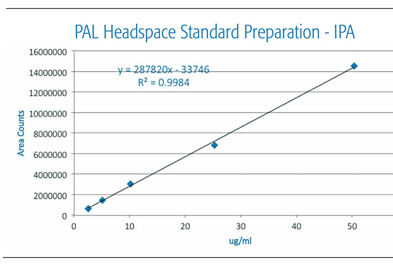
Figure 4: The standard curve for IPA headspace standards prepared by the PAL RTC automatically.
