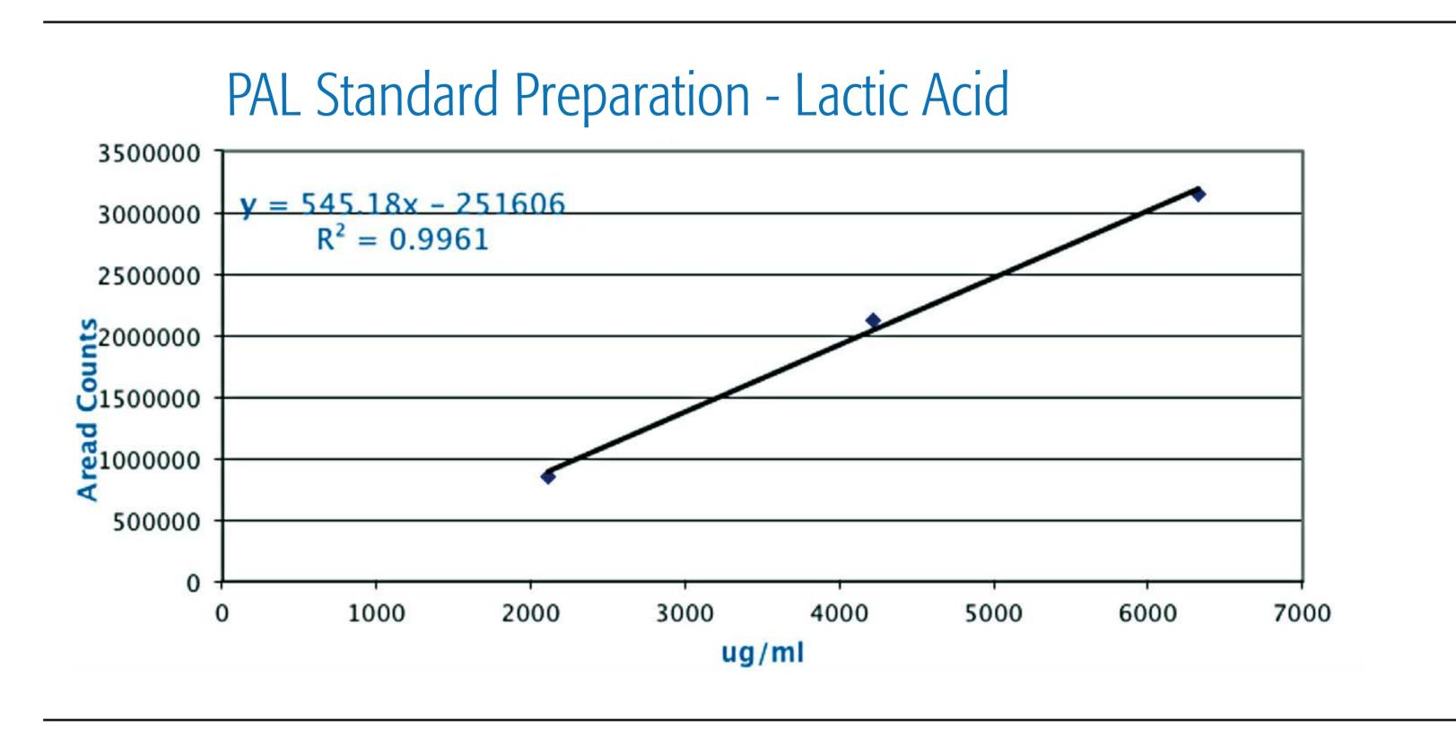
Figure 6: The standard curve for lactic acid standards prepared by the PAL RTC automatically.
