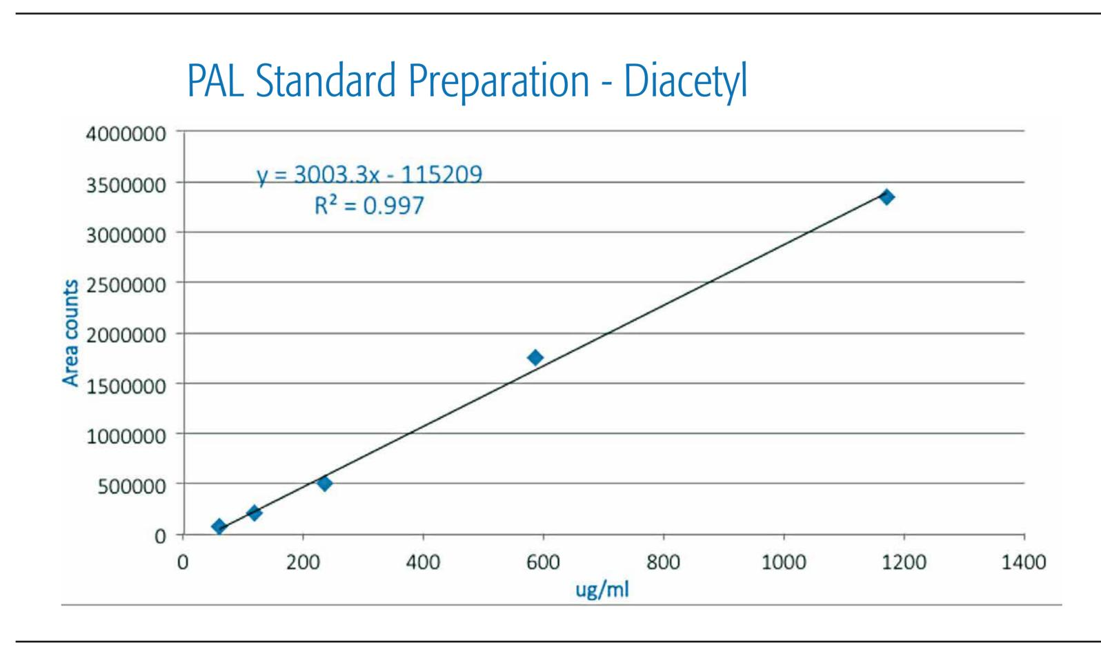
Figure 2: The standard curve prepared for diacetyl by the PAL RTC automatically.
